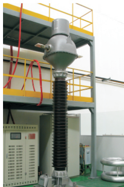
AGU-252 current transformer
